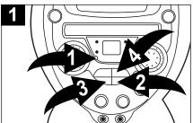
To repeat a single track, press the REPEAT button ① once; the REPEAT indicator will blink. Press the Skip/Search (►►I) ② or (►I) button ③ to select the specific track that you wish to repeat. When the desired track number blinks in the display, within five seconds, press the PLAY/PAUSE (►II) button ④ to begin playback. The specific track you selected will be repeated continuously.
